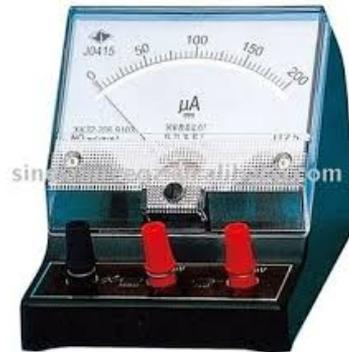
Mili ammeter and micro ammeter are using to measure current
